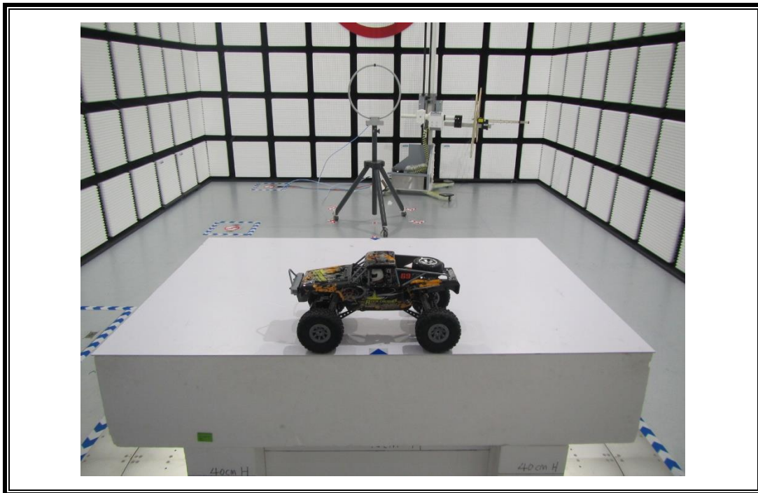
RADIATED RF MEASUREMENT SETUP (Below 30MHz)
