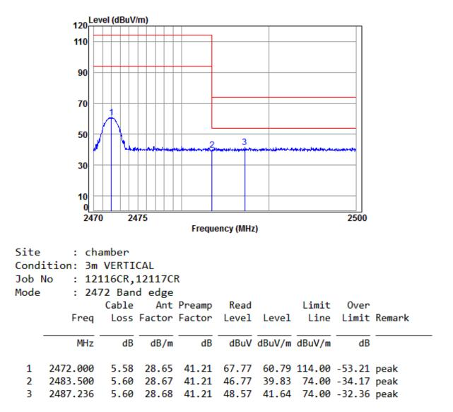
Mode:b; Polarization:Vertical; Modulation:GFSK; ; Channel:High
