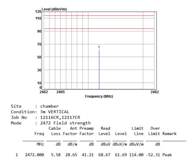
Mode:b; Polarization:Vertical; Modulation:GFSK; ; Channel:High
