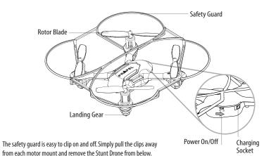
Note: Always have the safety guard attached when flying in T-Mode and Mode 1.
