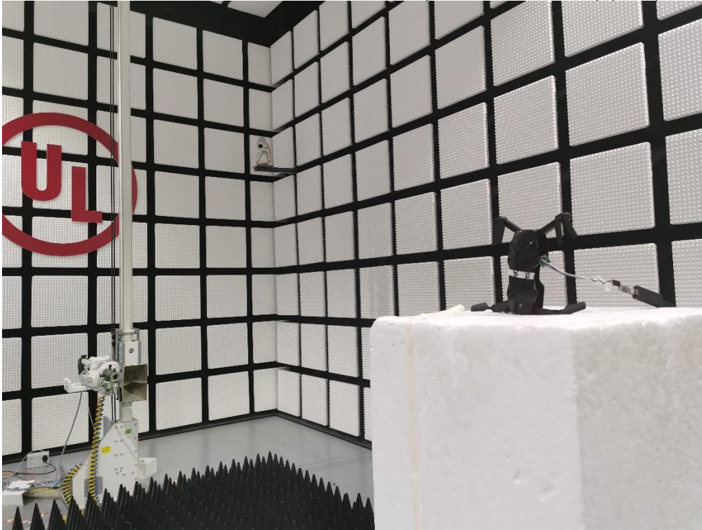
RADIATED RF MEASUREMENT SETUP (Above 1G – Y axis) (WiFi)
