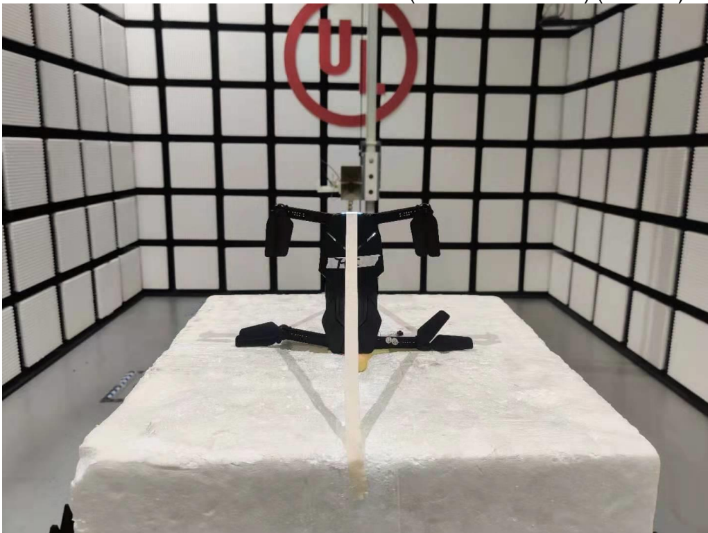
RADIATED RF MEASUREMENT SETUP (Above 1G – Y axis) (2.4 GHz)
