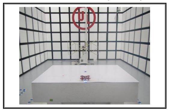
RADIATED RF MEASUREMENT SETUP (Below 30MHz)
