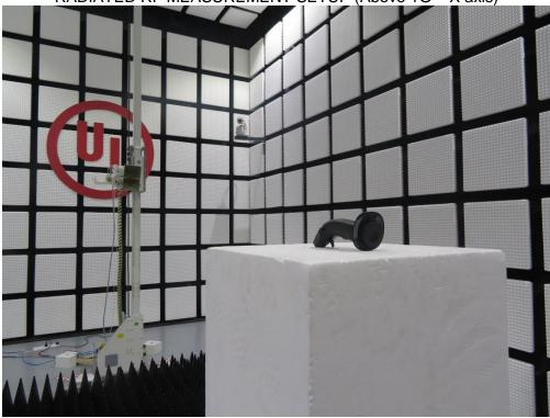
RADIATED RF MEASUREMENT SETUP (Above 1G - Y axis)
