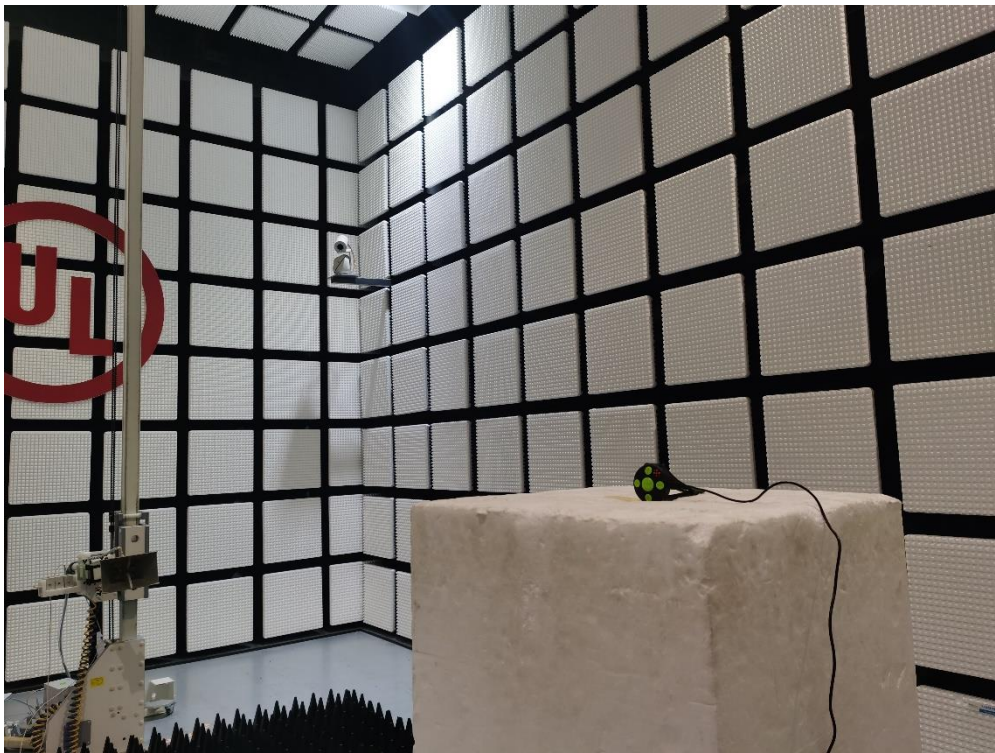
Radiated Disturbance Setup (Above 1 GHz – Y axis)
