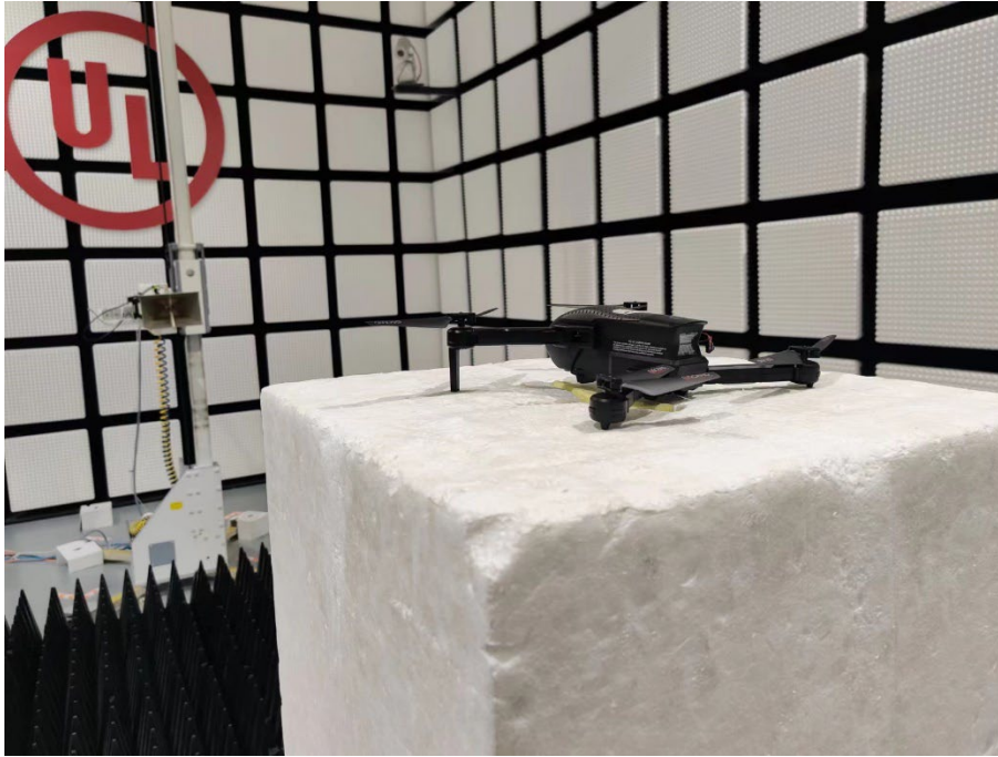
Radiated Disturbance Setup (Above 1 GHz – X axis)
