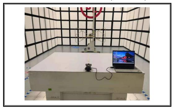
RADIATED RF MEASUREMENT SETUP (Below 30MHz)
