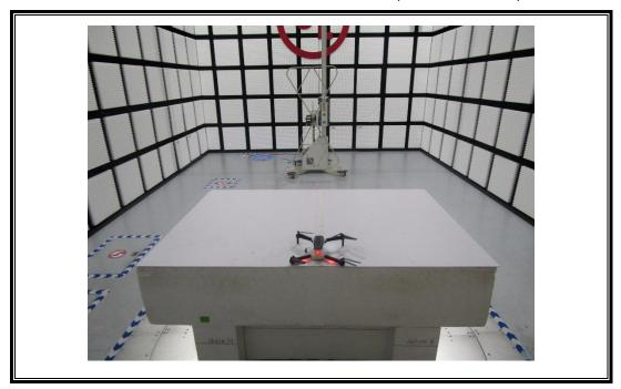
RADIATED RF MEASUREMENT SETUP (Below 30MHz)
