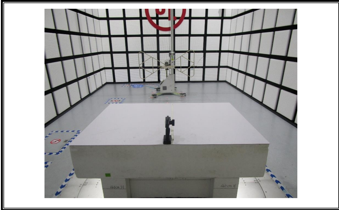
RADIATED RF MEASUREMENT SETUP (30MHz ~ 1 GHz)
