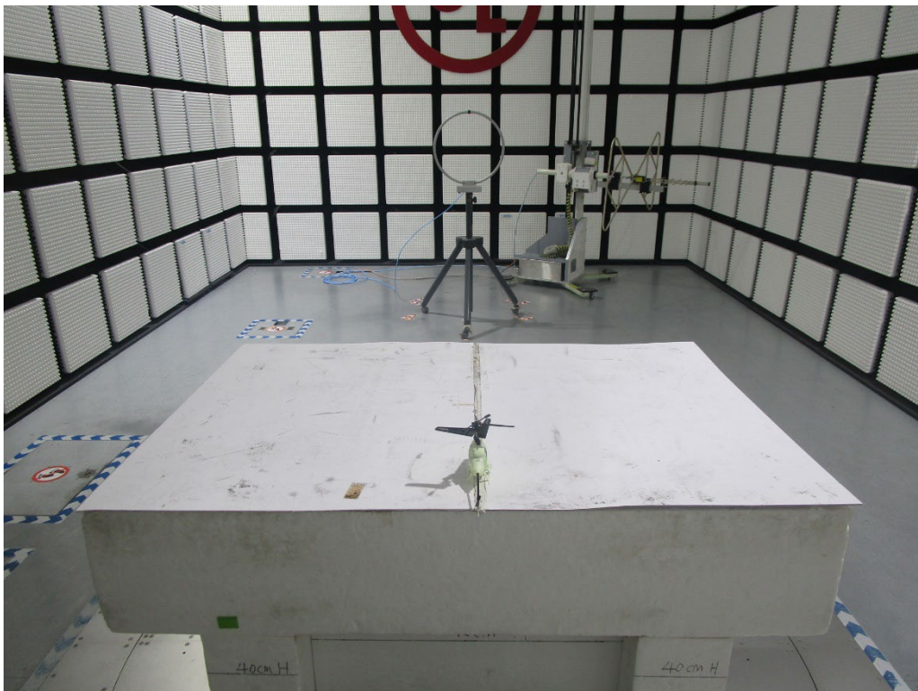
Radiated Disturbance below 30 MHz Test Setup For 2.4GHz SRD
