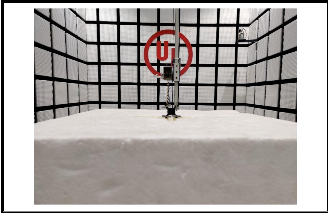
AC POWER LINE CONDUCTED EMISSIONS MEASUREMENT SETUP
