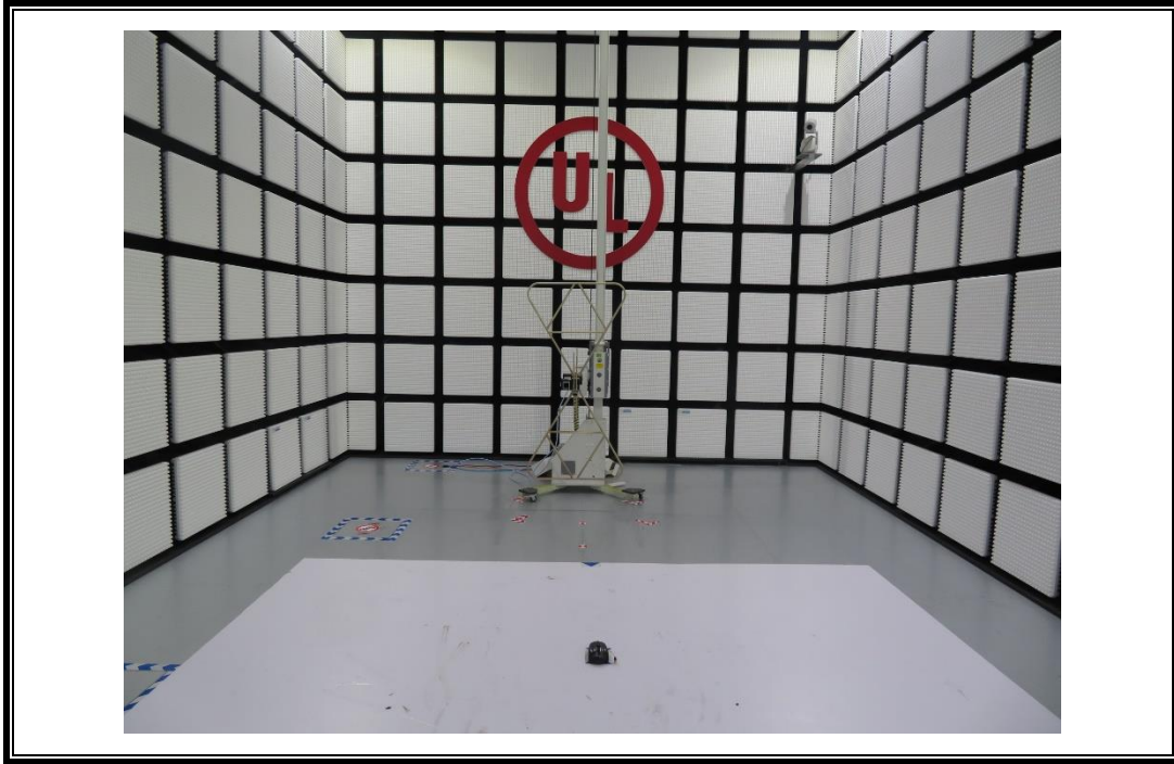
RADIATED RF MEASUREMENT SETUP (30MHz ~ 1 GHz)
