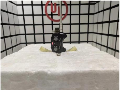
Radiated Disturbance Setup (Above 1 GHz – Worst Case)
