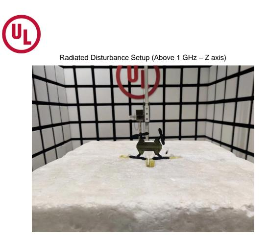
Radiated Disturbance Setup (Above 1 GHz – Worst Case)
