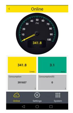
Please download the service app from the Google Play Store in case you need to have any settings changed on the S 415. The app is running on any Android system with Bluetooth supported. To change settings the app needs to scan the QR code on the calibration certificate at first. This ensures that only valid users can access the sensor settings. Follow the instructions in the service app.
