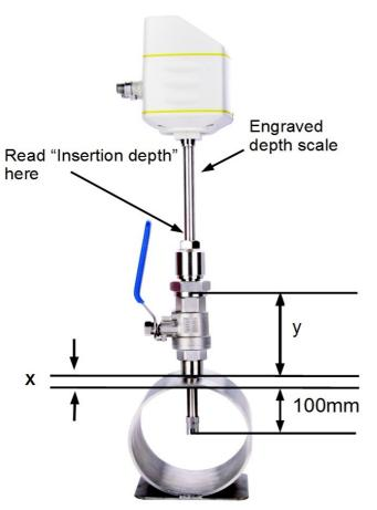
**Insertion depth** = x + y + 100x is the wall thickness of pipe y = length of the ball valve
