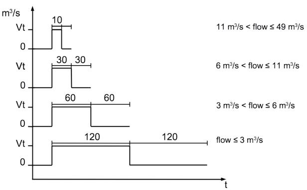
In case the flow rate is too high the S401 can not output the pulses with default settings (one pulse per consumption unit). For this the pulse can be set by our service software or a connected display to 1 pulse per 10 consumption units or 1 pulse per 100 consumption units. For example, if set to 1 pulse per 10 m<sup>3</sup>, the sensor will send one pulse each 10 m<sup>3</sup>. Example (1 pulse per 10 m<sup>3</sup>):
