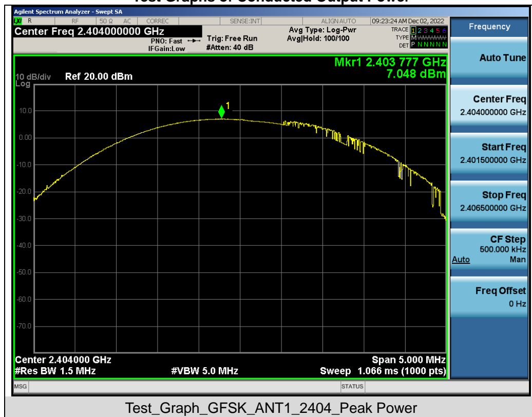
Test Graphs of Conducted Output Power
