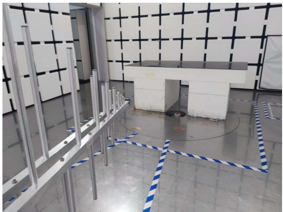
Radiation Emission Test Setup (30MHz to 1GHz)
