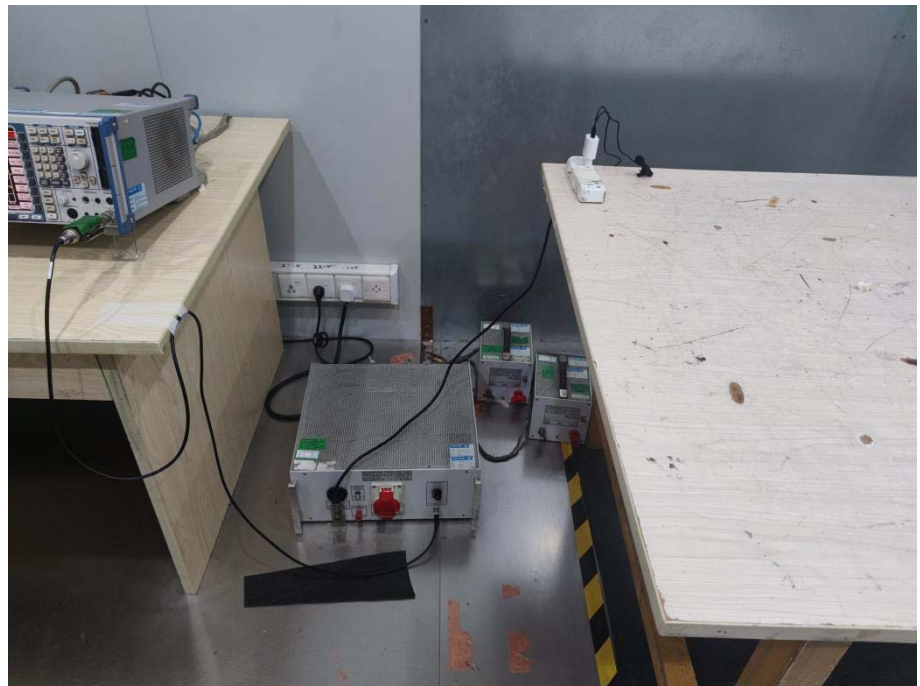
Conducted Emission Test Setup
