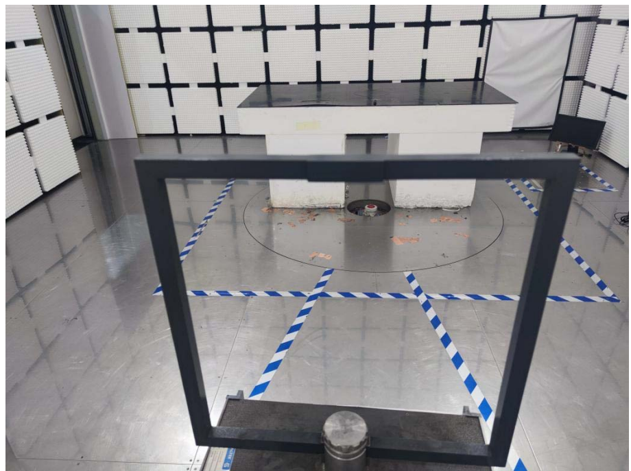
Radiation Emission Test Setup (Below 30MHz)
