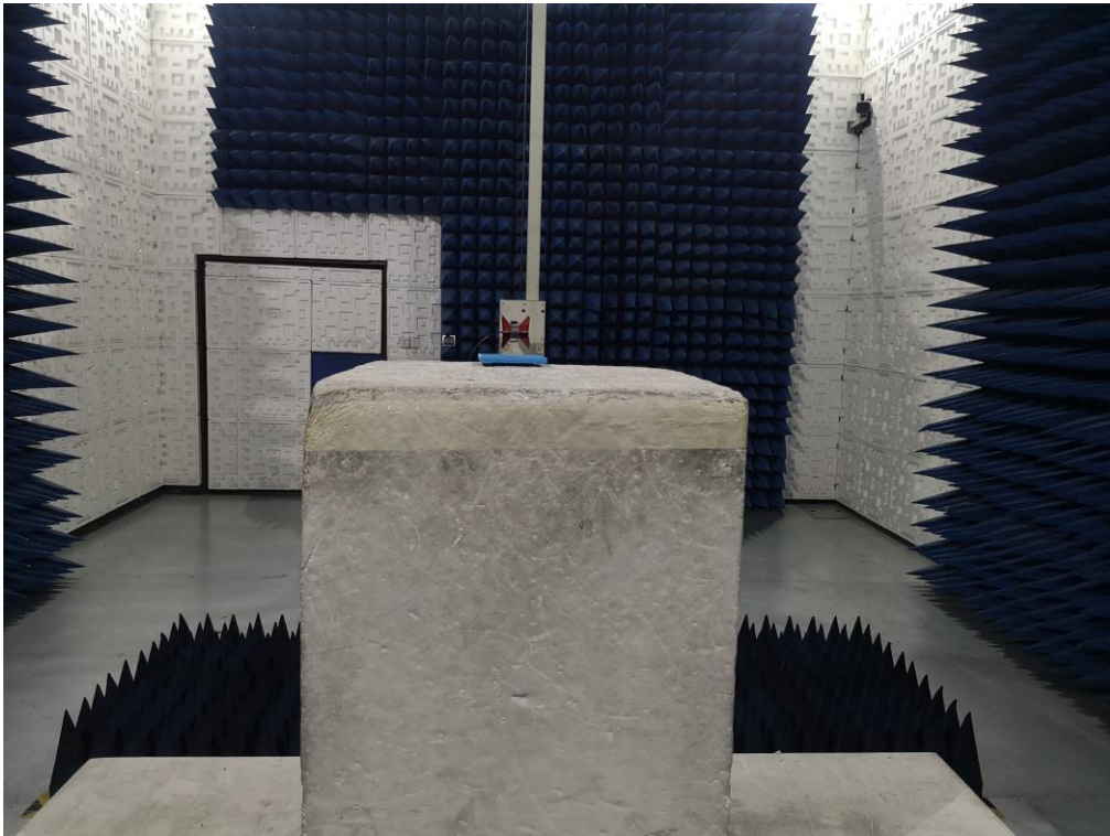
FCC RADIATED EMISSION TEST SETUP ABOVE 1GHZ
