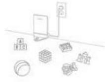
✗ Improper home base placement
