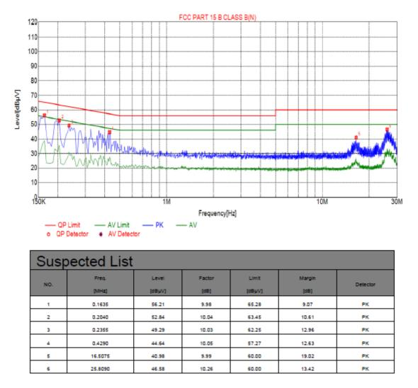
Remark: Transd = Cable lose + Antenna factor - Pre-amplifier; Margin = Limit – Level
