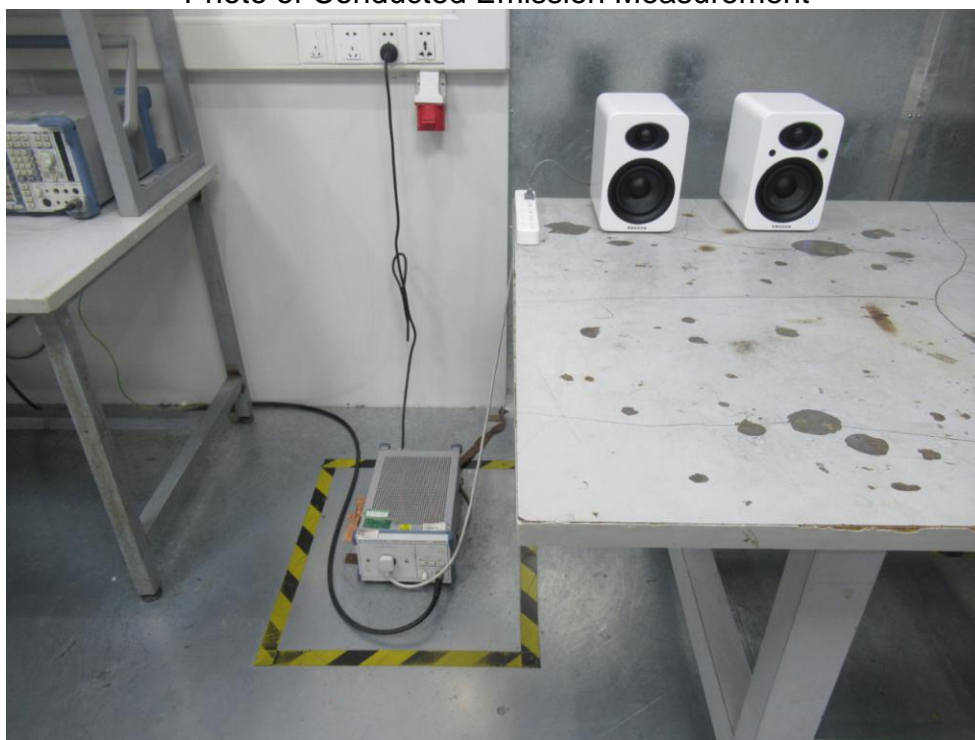
FCC ID: 2ASJK-S5 Photo of Conducted Emission Measurement
