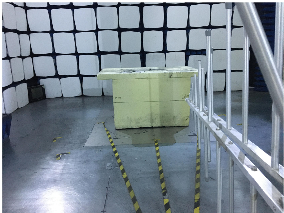
Radiation Emission Test Setup (30MHz to 1GHz)
