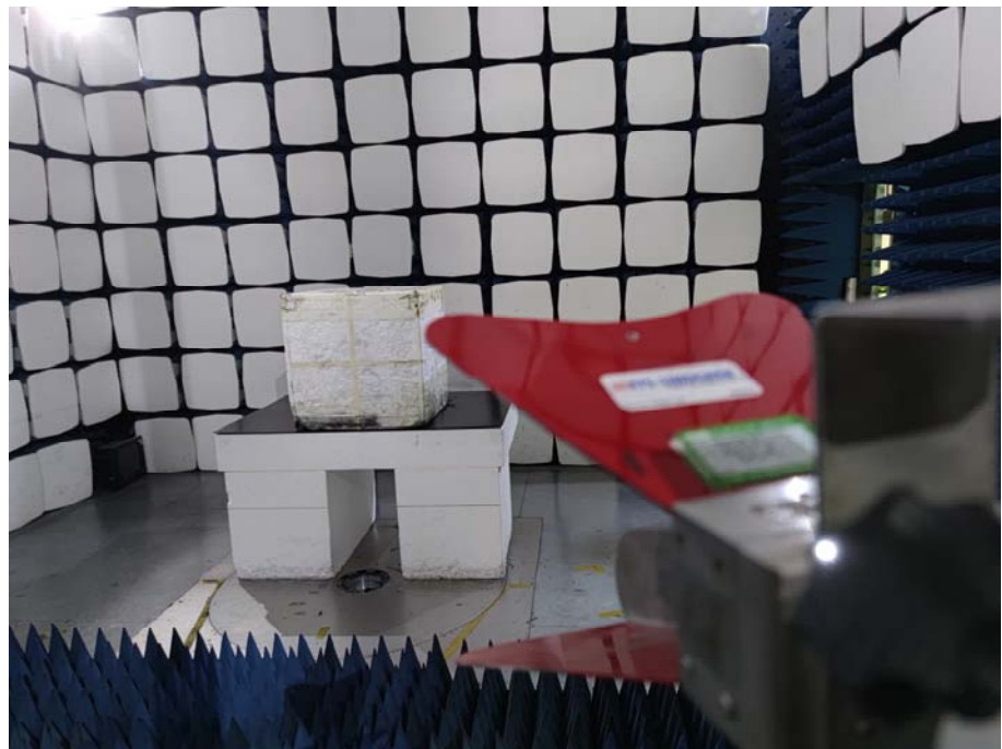
Radiation Emission Test Setup (1GHz to 18GHz)
