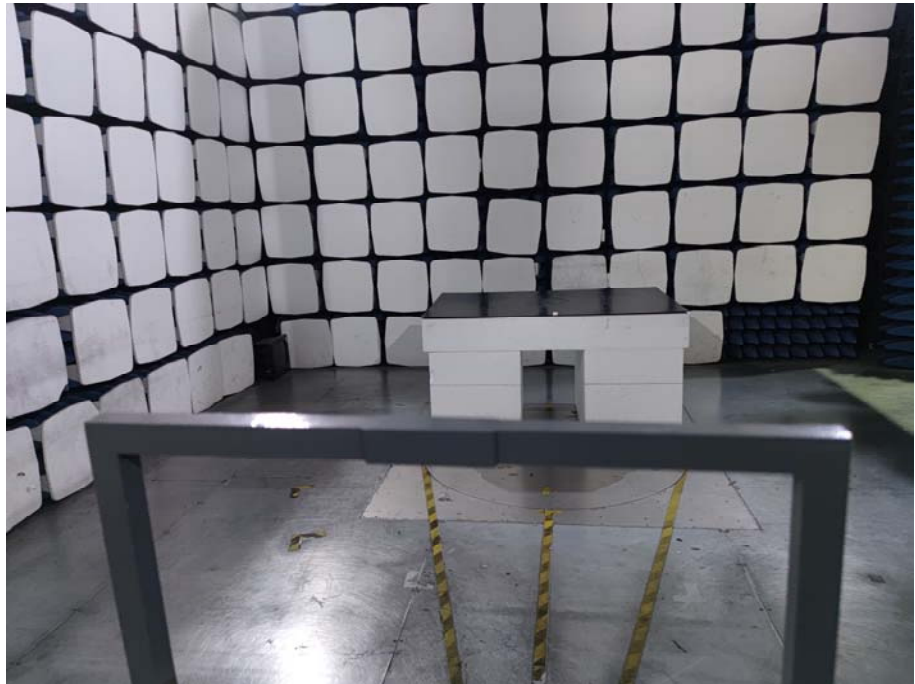
Radiation Emission Test Setup (Below 30MHz)
