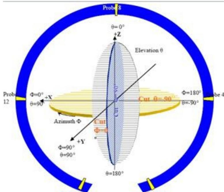
3D microwave darkroom testing coordinate system (back view)
