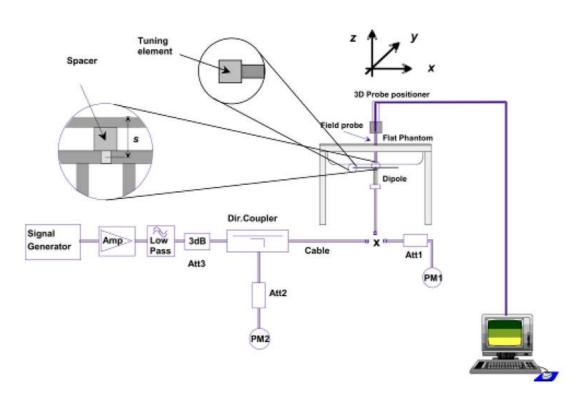
**System Verification Setup Block Diagram**
