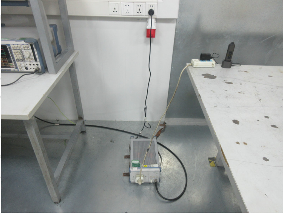
Photo of Conducted Emission Measurement
