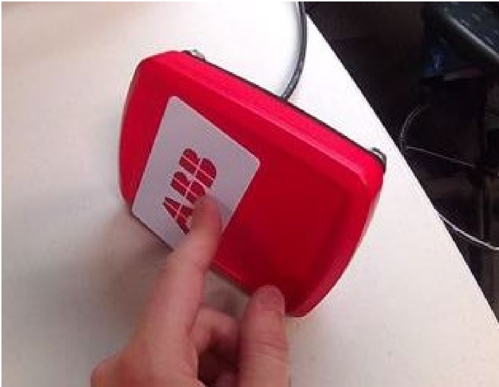
Using an RFID Tag to Enable WiFi Communications
