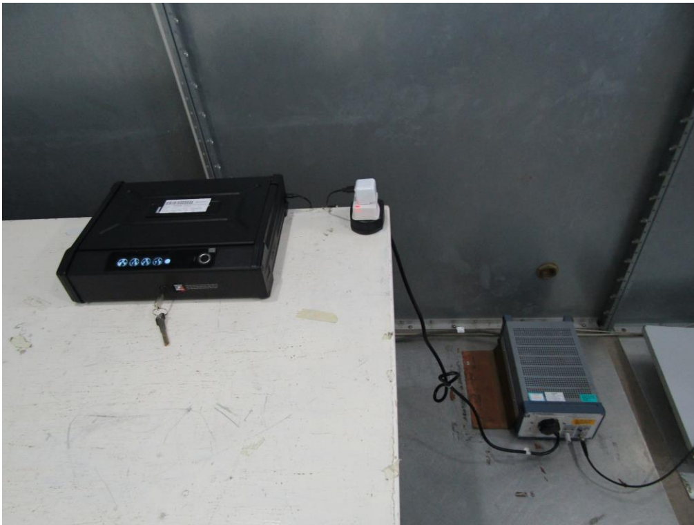
Measurement of Conducted Emission Test Set Up
