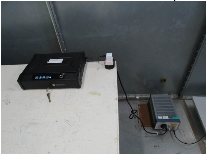
Measurement of Conducted Emission Test Set Up
