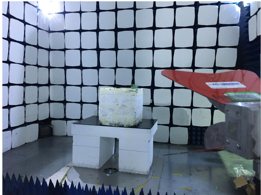
Radiation Emission Test Setup (1GHz to 18GHz)
