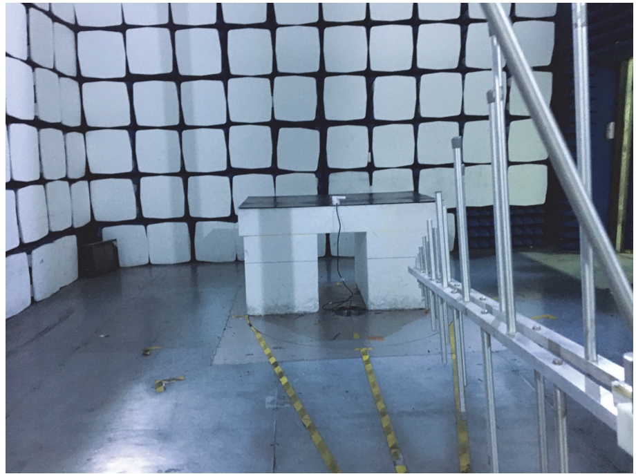
Radiation Emission Test Setup (30MHz to 1GHz)
