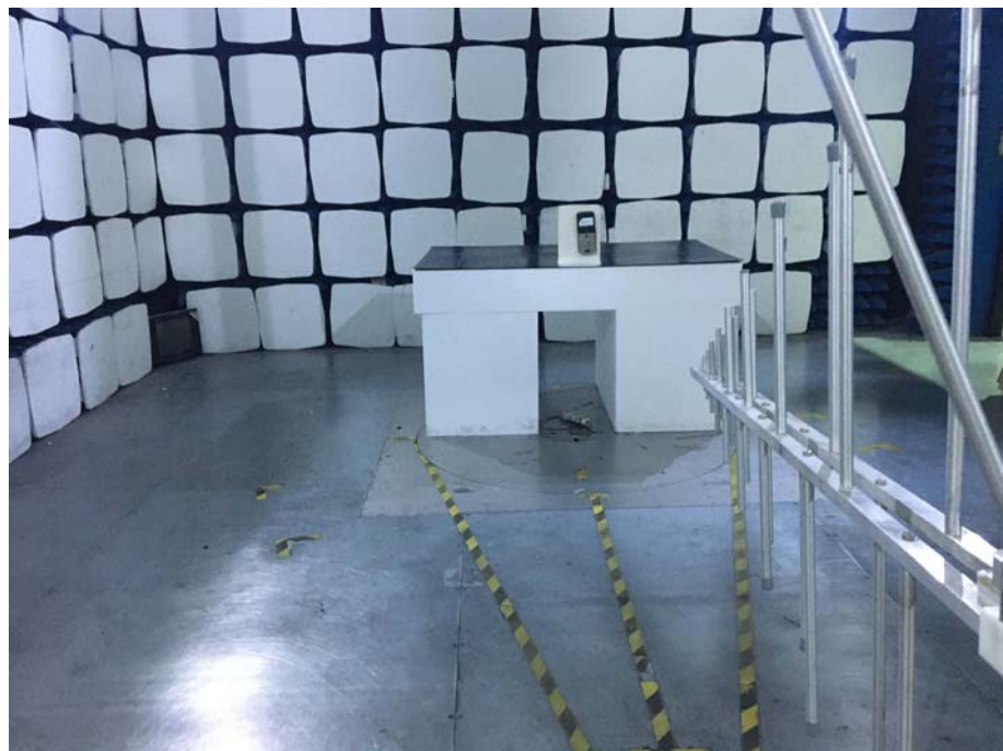
Radiation Emission Test Setup (30MHz to 1GHz)
