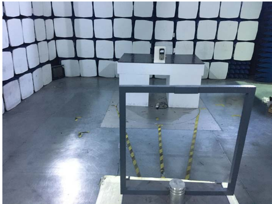
Radiation Emission Test Setup (Below 30MHz)
