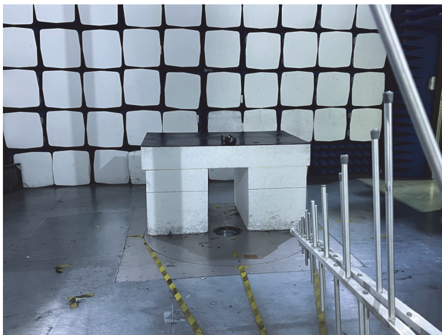
Radiation Emission Test Setup (30MHz to 1GHz)
