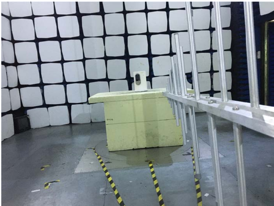
Radiation Emission Test Setup (30MHz to 1GHz)
