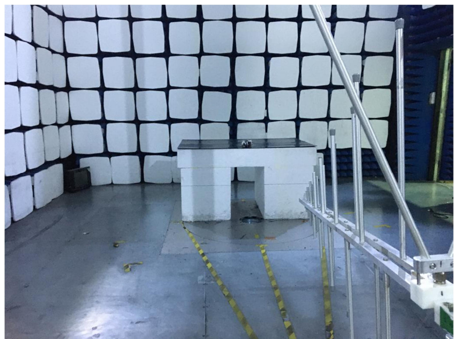
Radiation Emission Test Setup (30MHz to 1GHz)
