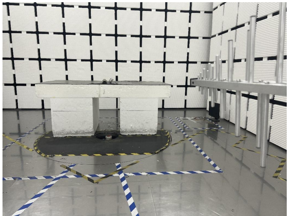
Radiation Emission Test Setup (30MHz to 1GHz)
