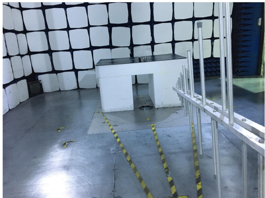
Radiation Emission Test Setup (30MHz to 1GHz)
