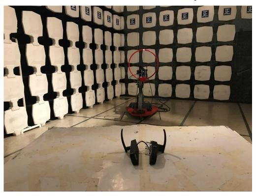
Measurement of Radiated Emission Test Set Up
