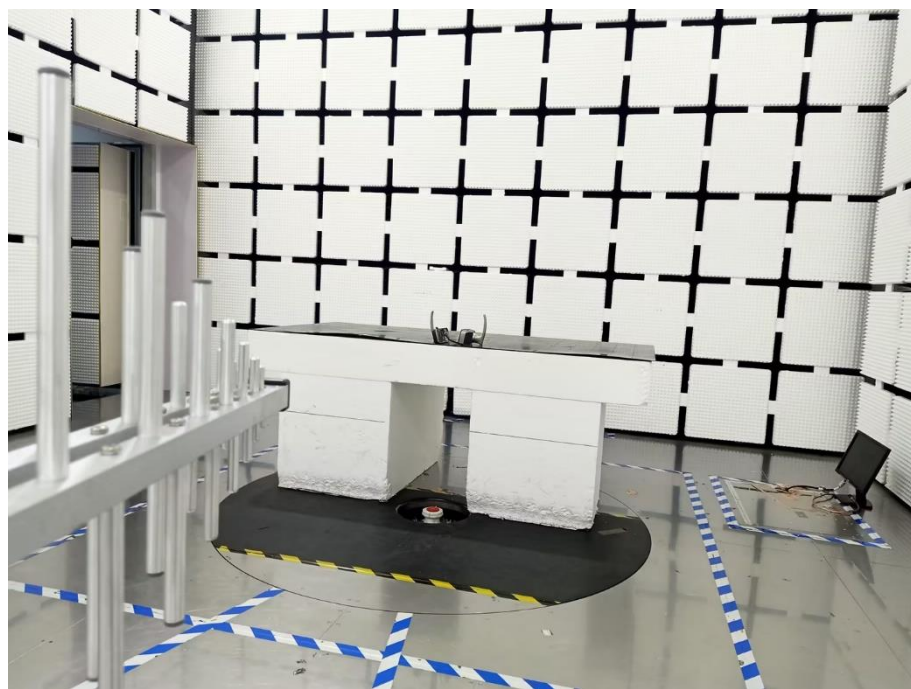
Radiation Emission Test Setup (30MHz to 1GHz)
