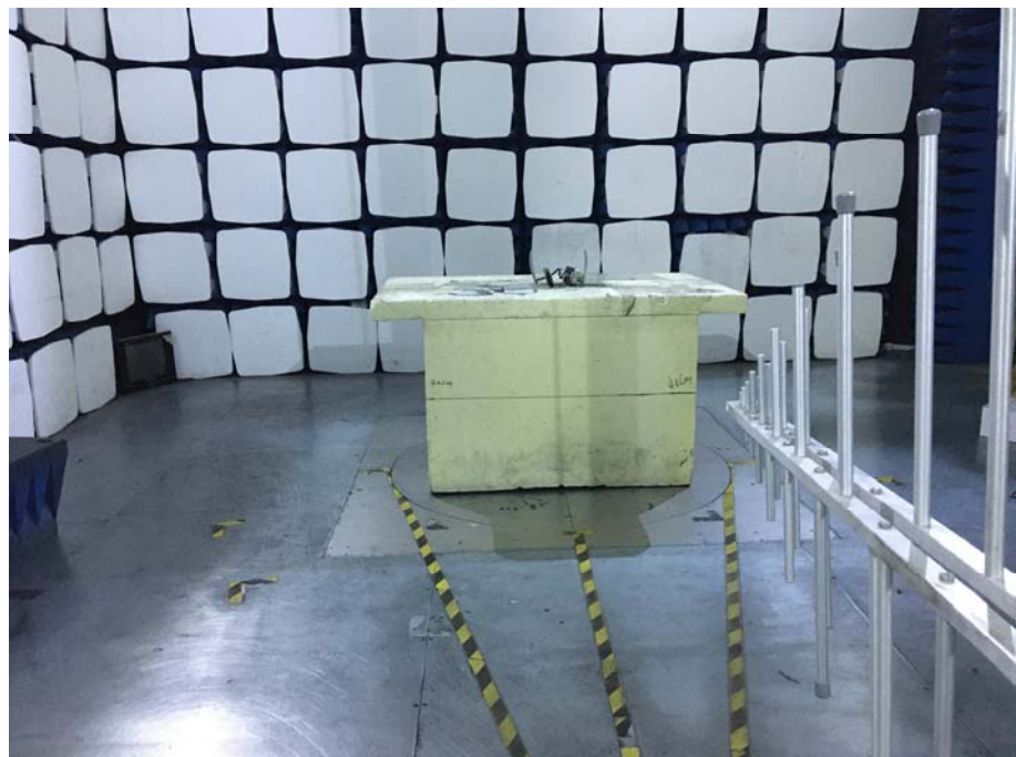
Radiation Emission Test Setup (30MHz to 1GHz)
