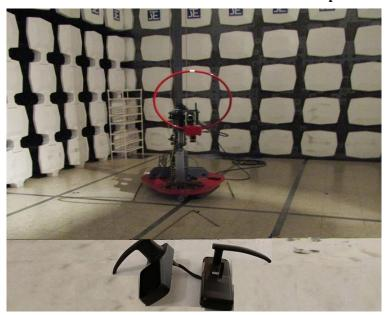
Measurement of Radiated Emission Test Set Up
