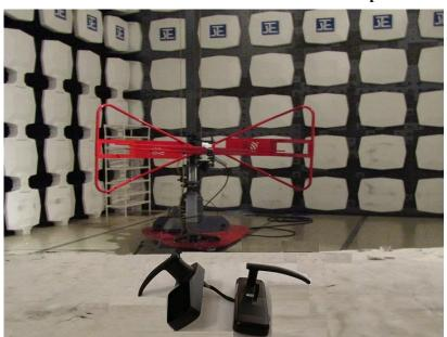
Measurement of Radiated Emission Test Set Up
