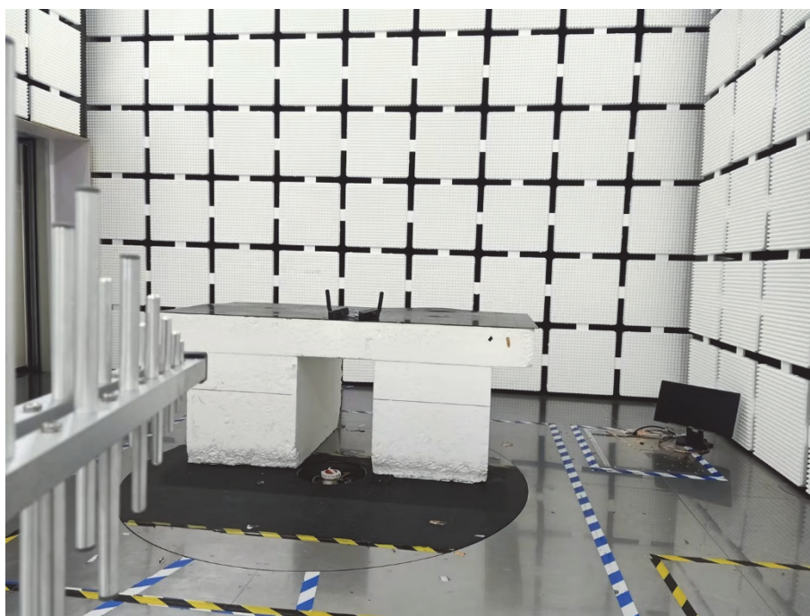
Radiation Emission Test Setup (30MHz to 1GHz)
