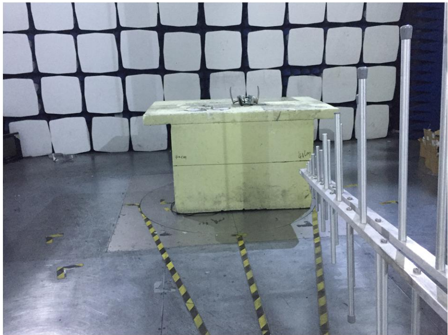
Radiation Emission Test Setup (30MHz to 1GHz)
