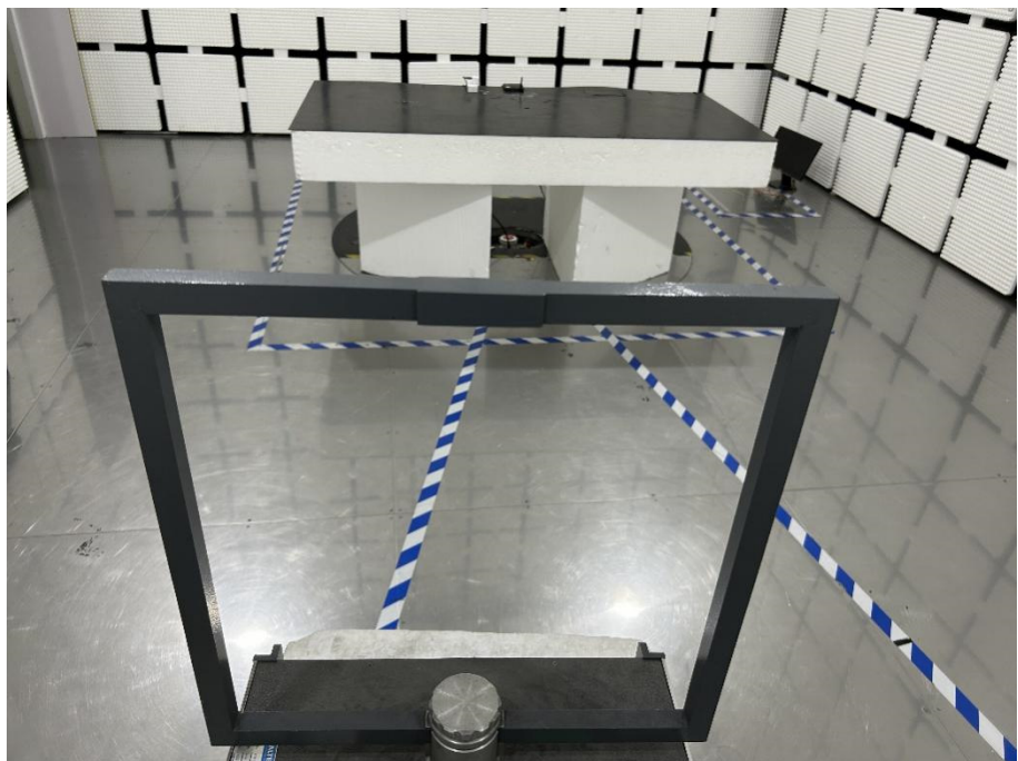
Radiation Emission Test Setup (Below 30MHz)
