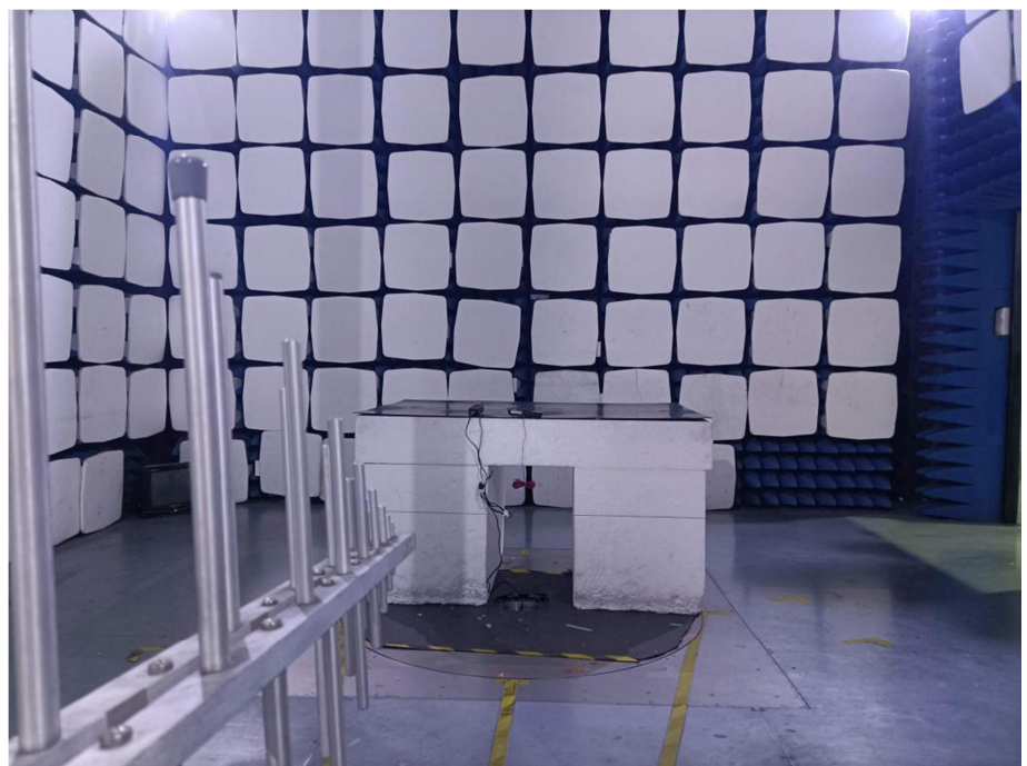
Radiation Emission Test Setup (30MHz to 1GHz)
