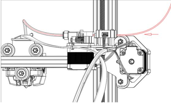
Cut the filament tip pointy, hold down the extruder handle, and push the filament into the extruder into the filament tube at the same time.
