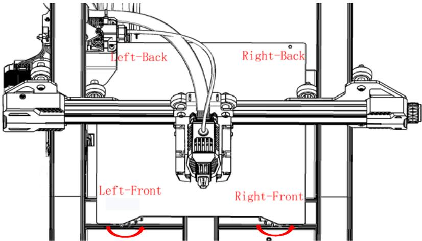
When the thumbscrew is turned clockwise, the bed will rise, and counterclockwise, the bed will descend.
