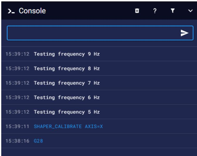
Note: it will vibrate in the X axis at this time. Please observe the printer first to ensure that the vibration is not too strong.
