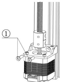
**Note:** Install the T8 lead screw into its copper nut.
