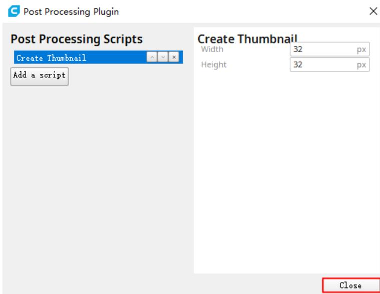
The default resolution of CURA is 32\*32 (you can adjust it according to the display effect).
