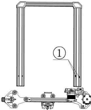
①: Pay attention to the direction, there are two M4 holes. The POM wheels on both sides are aligned with the Z-axis aluminum part. If it is too tight or too loose, the eccentric nut can be adjusted with a wrench so that the POM wheels on both sides of the Z-axis do not shake and are not too tight.
