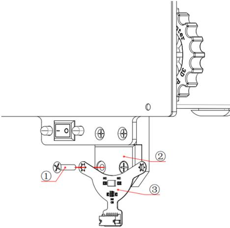
Install the left fixing hole of the ADXL345 module in the position where you just removed the screws.
