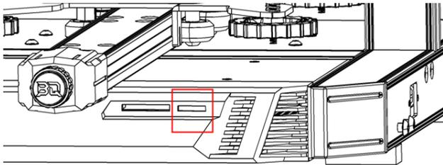
Insert Micro SD and power the machine on again.
