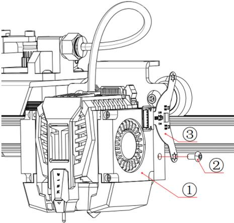
Install the fixing hole of the lower end of the ADXL345 module in the position where the screw was just removed.
