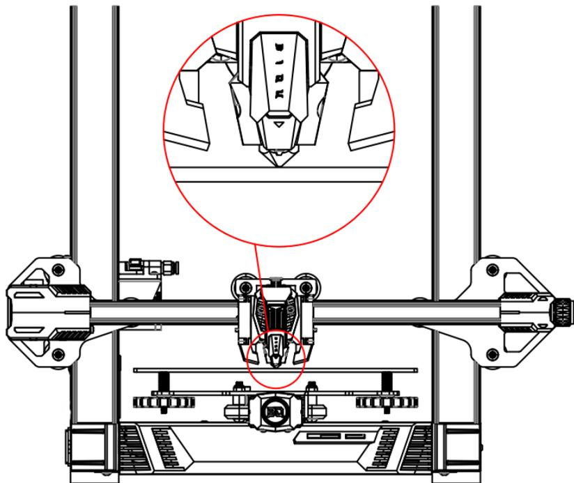
Make sure the distance between the bed and the nozzle is between 0 and 0.1mm.
