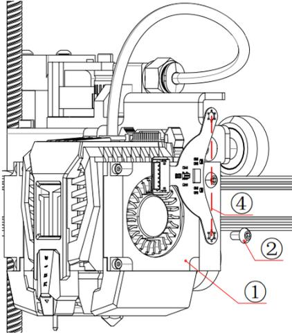
Adjust the position and fix it with M3x6 screws.
