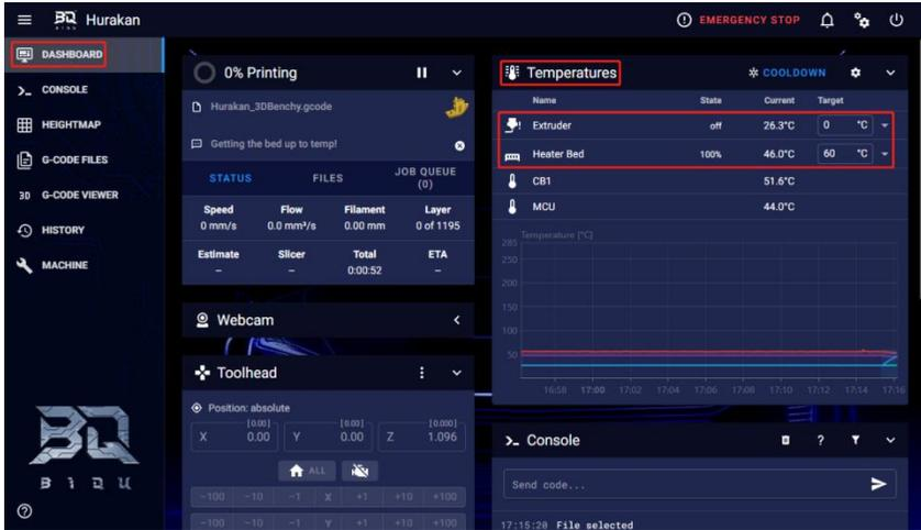
The print will start after the components reached the printing temperature.
