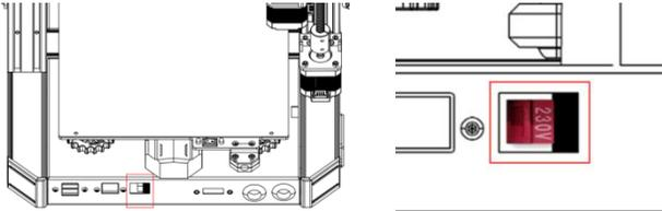
Voltage Mode: 115V(Switch to right, you will see 115V marked on the switch), corresponding to Household Voltage: 100—120V;
