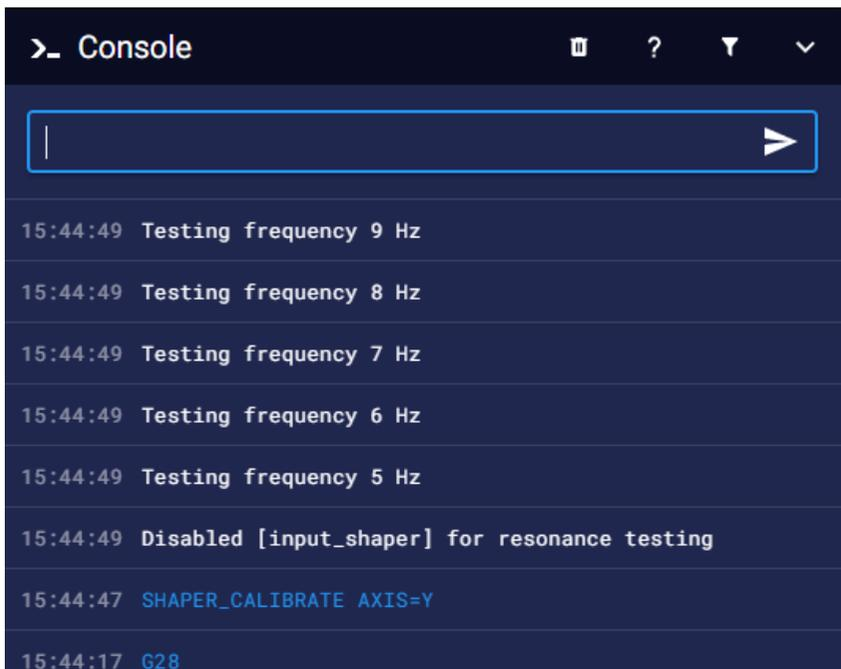
Note: it will vibrate in the Y axis at this time. Please observe the printer first to ensure that the vibration is not too strong. After calibration, enter the save code: **SAVE\_CONFIG**
