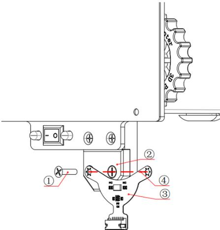
Adjust the position and fix it with M3x10 screws.
