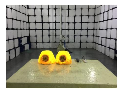
Radiation Emission Test Setup (1GHz to 18GHz)
