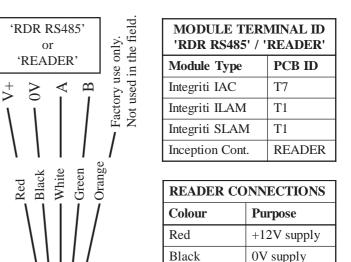
Orange Factory only To extend the length of the Reader pigtail Reader Cable. cable, twisted pair cable is used as follows: Data A and Data B Pair 1. V+ and 0V. Pair 2.
